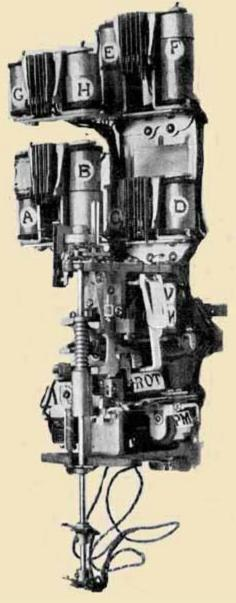
Left: U.S. switch, 1912. The contact bank has been removed from the base of the switch.
